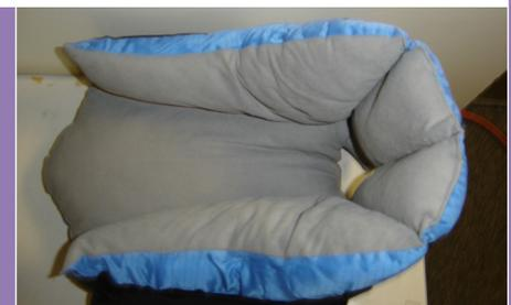
Two samples of three different styles of boot construction were tested: open-celled ventilated foam, air bladder, and pillow. The microclimate was continuously monitored via temperature and humidity sensors.
